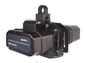
The **Apex Hoist** is available in both 500kg and 1250kg versions capable of speeds of 30m/min and 12m/min respectively. It is equipped with two silent, monitored brakes, dual encoders and an integral loadcell all of which enable SIL3 operation and compliance with DIN56950 and BS7905.
