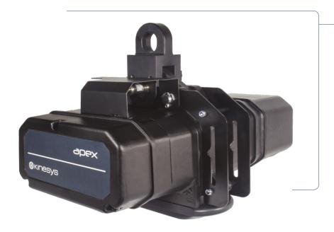
The **Apex hoist** range offers both a 500kg (1200lb) and a 1250kg (2750lb) option. The hoists have maximum speeds of 500mm/s (100ft/min) and 200mm/s (40ft/min) respectively in compact packages while still maintaining the highest safety standards suitable for movement over people in show situations.
