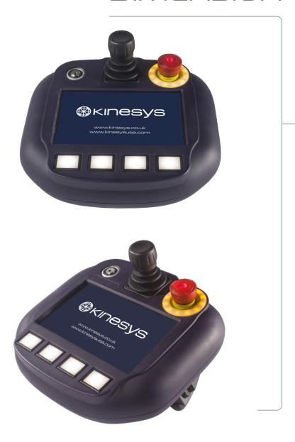
The Dimension range of operator controls starts with the **Dimension pendant**. It meets perfectly the demand for a fully capable handheld device with an intuitive easy to use interface. Designed in-house by Kinesys the custom enclosure is ergonomic and compact while still including all the hardware required for both rigging and show operations.
