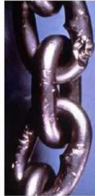
HEAT DAMAGE & NICKS AND GOUGES
